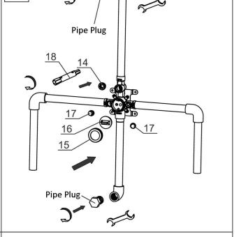
Install piping and elbows to shower and bath outlets. Connect the water supplies. Apply sealant tape to all threaded connections.
