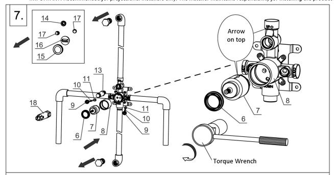
Remove the pipe plugs and components 14, 15, 16 and 17. Install components 11, 10, 9, 13, 8, 7 and 6. When installing 7 (Cartridge), make sure the arrow is on top pointing toward the valve. Use a torque wrench (10-12 Nm) to assemble.
